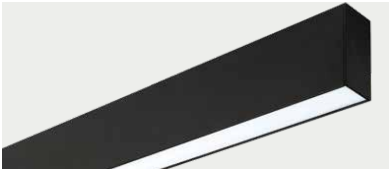
34mm LED profile luminaire, made of an extruded aluminium, power-coated with fine sandy finish. Designed for ceiling/pendant/trimless/recessed mounting, providing direct light emission through PMMA diffuser. Luminaire equipped with the latest generation of well known LED boards with small color tolerance.
