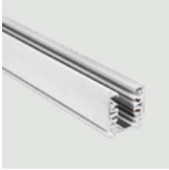
Dimensions Description Color Color L: 400cm W: 3.2cm H: 3.5cm Square Track Surface 100-240V Black / Code 19400-4M White / Code 19401-4M
