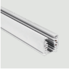
Dimensions Description Color Color L: 300cm W: 3.2cm H: 3.5cm Square Track Surface 100-240V Black / Code 19400 White / Code 19401
